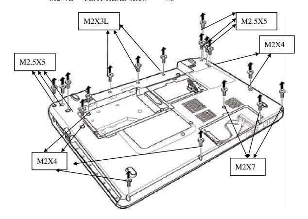
Figure 4-15 Removing the screws on bottom case
